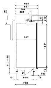
ED Remote electrical connection RO Refrigerant Outlet
